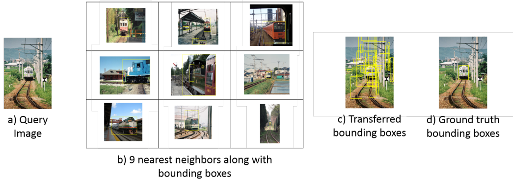
Figure 1. For a query image (a), our system finds the top matches (nine are shown here) (b) Using SIFT flow matching algorithm [9], the bounding boxes of the top matches are transferred to the input image, as shown in (c). For comparison, the ground-truth user annotation of (a) is shown in (d).
