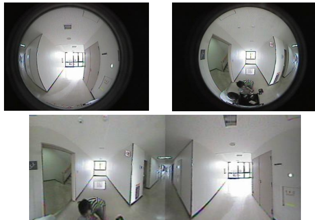
Figure 1: Examples of full-view images. Top: Two half scenes captured by fisheye camera. Bottom: A panorama view.
