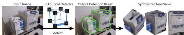
Figure 1. Given a single-view input image, our goal is to detect the 2D corner locations of the cuboids depicted in the image.
