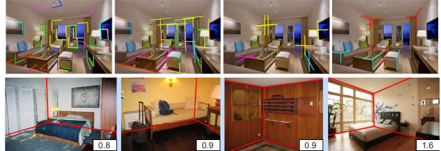
Figure 3. On the top row, we show prominent junctions such as L, T, X and Y ordered from left to right. On the bottom we show a few top scoring layouts along with the pixel-misclassification error shown on bottom right.
